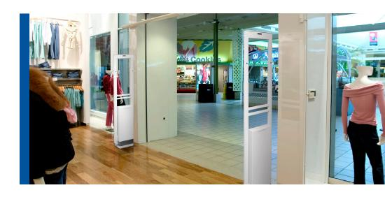
sensors also enable a "power-on-demand" feature that puts the system into low-power standby mode during periods of low or no traffic activity to reduce power consumption up to 90%.
