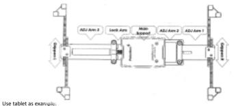
1,Centre the tablet on the Main Support horizontally. Grip the tablet in width with *Grippers R*, screw down the R Grippers here. Adjust Grippers L to have same tick marks as Grippers R, screw down L Grippers here.
