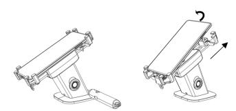
Plug Key into the key port in the post. In 2~3 seconds the Lock arm shall popup and release the phone/tablet along with the LEDs blinking on post and key.
